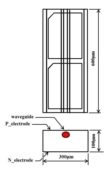
O P-electrode and N-electrode are both gold pads.
