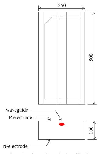
P-electrode and N-electrode are both gold pads.
