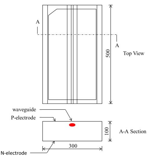
◎ P-electrode and N-electrode are both gold pads.
