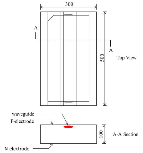
P-electrode and N-electrode are both gold pads.
