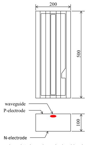
P-electrode and N-electrode are both gold pads.
