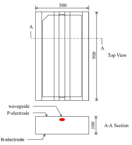
P-electrode and N-electrode are both gold pads.
