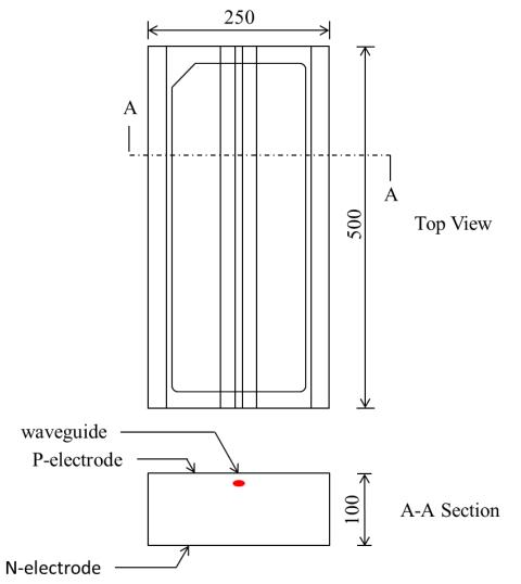
P-electrode and N-electrode are both gold pads.
