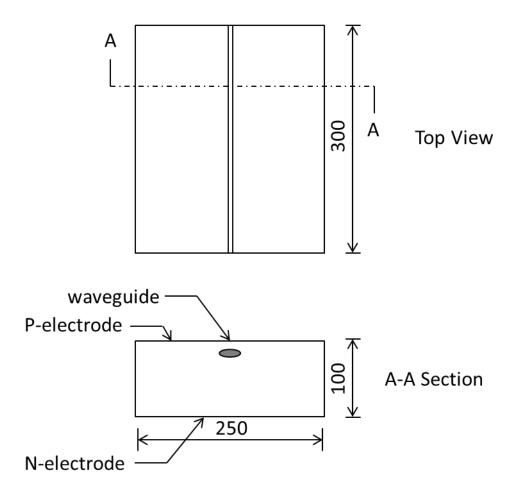
P-electrode and N-electrode are both gold pads.
