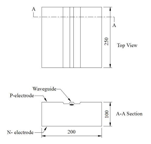
P-electrode and N-electrode are both gold pads.
