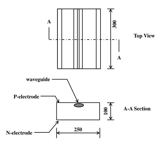
P-electrode and N-electrode are both gold pads.
