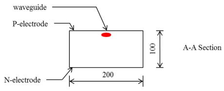
P-electrode and N-electrode are both gold pads.
