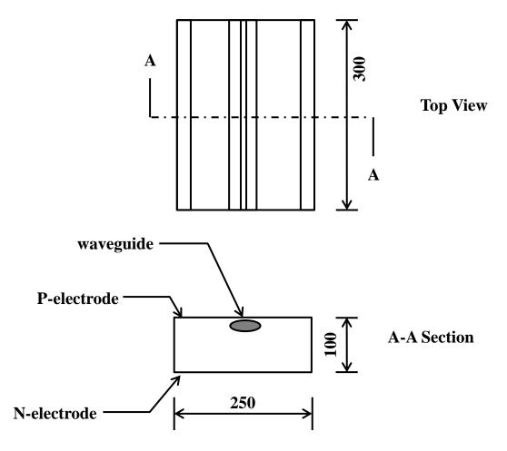
P-electrode and N-electrode are both gold pads.
