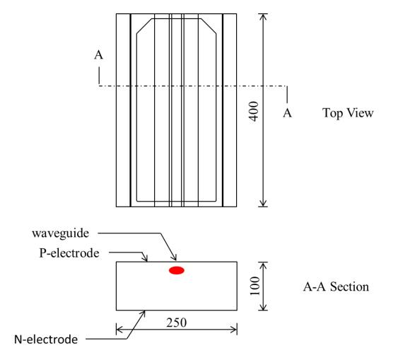
P-electrode and N-electrode are both gold pads.
