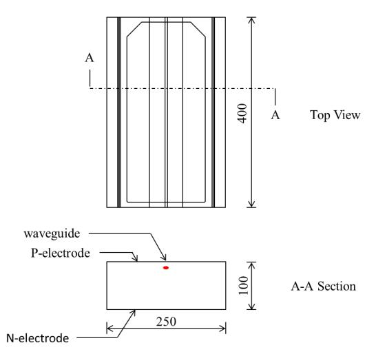
P-electrode and N-electrode are both gold pads.
