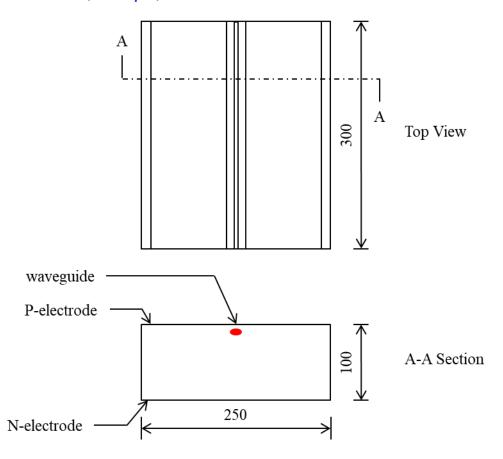
P-electrode and N-electrode are both gold pads.
