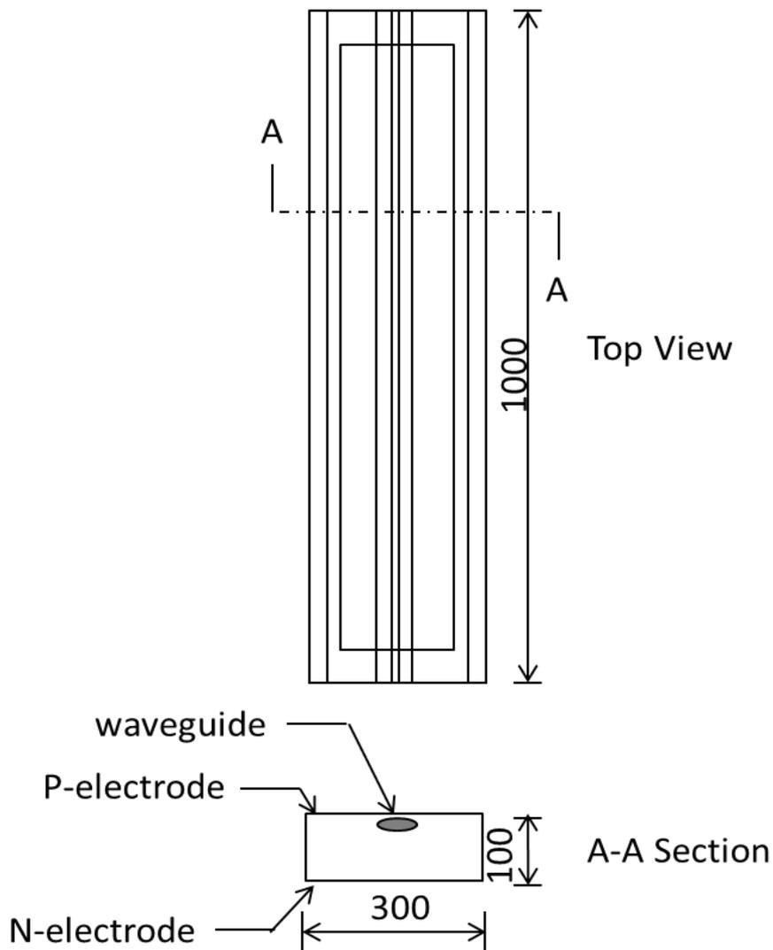
**P-electrode and N-electrode are both gold pads.**
