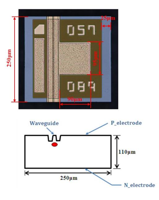
O P-electrode and N-electrode are both gold pads.
